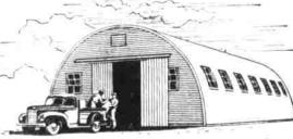
QUONSET 36-36 feet wide by any length desired. in sections of 20 feet. Each standard end wall is esprend with two steel windows, sliding steel doors adjustable centilating louvers. Side window and solid end walls are also available.
