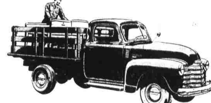
MEDIUM-DUTY DE LUXE STAKE* Model 3609—125 1/4-inch wheelbase, Maximum G.V.W. 5,800 lb. Other models available up to 161-inch wheelbase and 16,000 lb. G.V.W.
