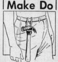
TO CARRY a hammer while working on a ladder, roof or scaffold, bend a piece of heavy wire over your belt and around the hammer to form a handy holder. (Popular Mechanics)
