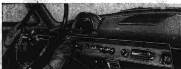
New Auto-Dial Instrument Panel is a safety dividend with speedometer placed high on the panel for easier reading. Warning lights tell when generator is discharging or oil pressure falls too low.
