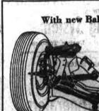
With new Ball-Joint Front Suspension
