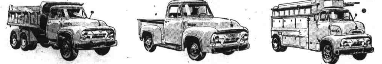
New Ford Master-Guide Power Steering is standard equipment on this new Ford F-100 factory-built 6-wheeler. GVW 40,000 lbs. 170-h.p. Cargo King V-8. New Power Brakes on this new Ford F-100 Pickup, at low extra cost. With 130-h.p. V-8 it's the world's most powerful Pickup! GVW 4,800 lbs. Deluxe Cab shown (extra cost). New Cab Forward giant Ford C-900 Big Job. GVW 27,000 lbs., GCW 55,000 lbs. Hauls 35-ft. trailers legally in every state. 170-h.p. Cargo King V-8.
