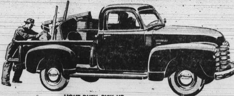
LIGHT-DUTY PICK-UP Model 3104—116-inch wheelbase, Maximum G.V.W. 4,600 lb. Other models available: 3604—125 1/4-inch wheelbase, Maximum G.V.W. 5,800 lb; 3804—137-inch wheelbase, Maximum G.V.W. 6,700 lb.
