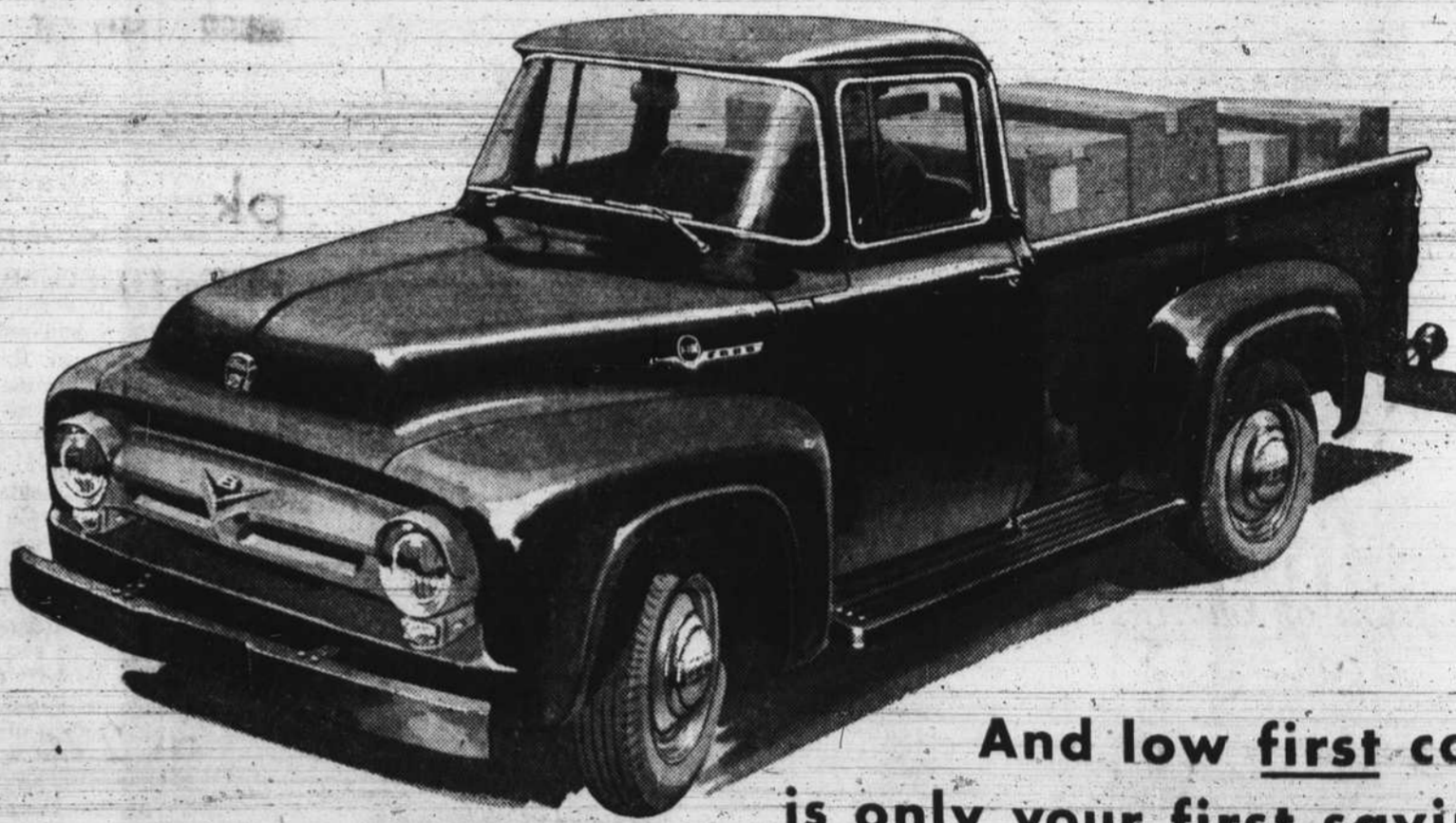
Ford's F-100 pickup with 8-ft. box is the biggest in the half-ton field—up to 19 cu. ft. more loadspace than the others. Regular 6 1/2-ft. box with a full 45 cu. ft. capacity also available.
