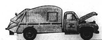
NOW % TON MORE GVW-Economy champ in its class, Ford F-700 is now rated at 21,000 lbs. GVW with heavy-duty rear springs. 140h.p. Short Stroke V-8. Single or electric-shift 2-speed rear axle.
