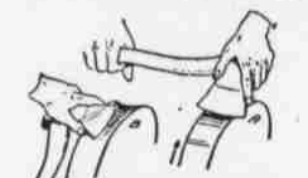
Correct way (A) to hold axe in grinding. Wrong way (B) makes groove in grindstone and spoils it.
