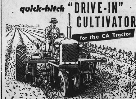
The Allis-Chalmers "drive-in" system eliminates heavy lifting and blocking up ordinarily required for frontmounted tools. You just drive your tractor into the frame and bolt it on.
