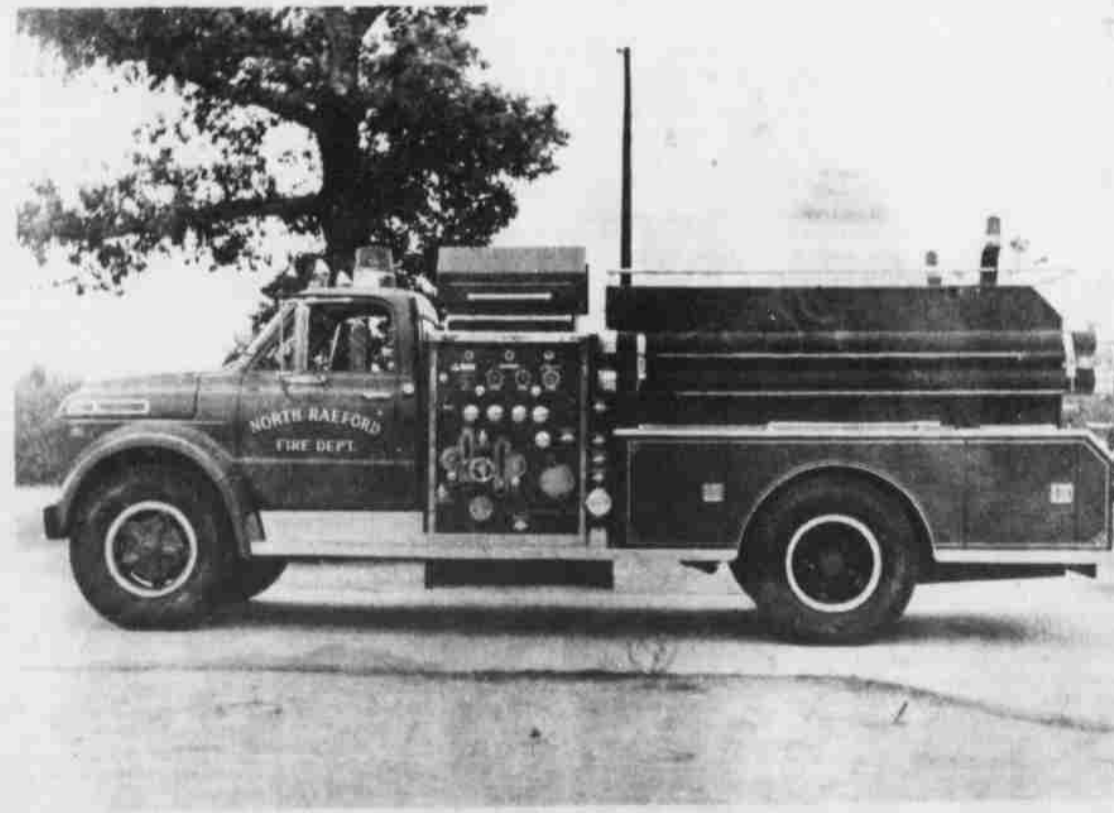
PRIDE OF NORTH RAEFORD - This is the new John Bean fire truck which was recently purchased by the North Raeford Volunteer Fire Department. The machine can deliver up to 9,000 pounds of pressure per square inch and features a screen device which will produce a dense and highly effective "fog" of water for combating fires.
