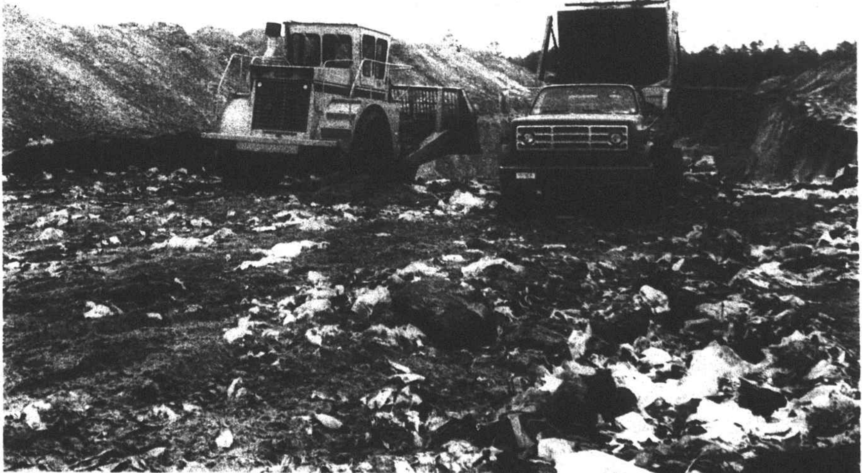
Compactor (left) and truck unloading garbage.
