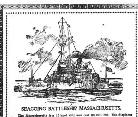
chusetts is a 15 knot ship and cost \$3,020,000. 188 tons of water, has 9,000 horsepower and carries four 13 inch,
