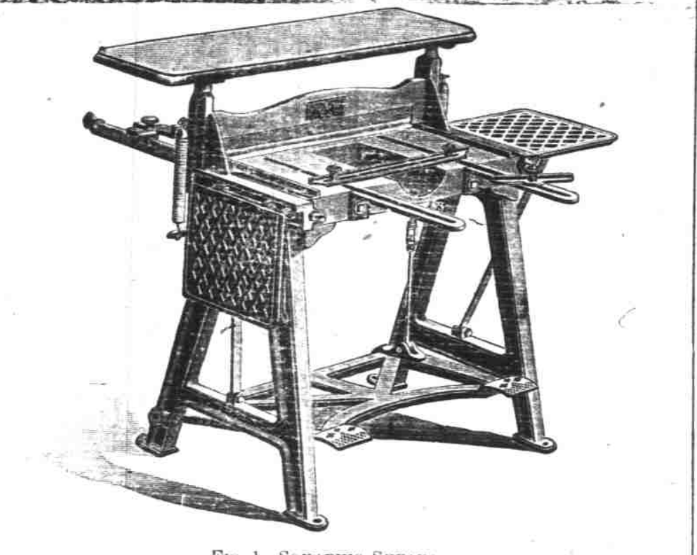
FIG. 1—SQUARING SHEARS. This machine is worked by foot power, and is adjustable for any ordinary size of can. It costs $40.
