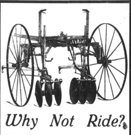
Any one who has used the ordinary type of Disc Cultivators, where the Discs have to be guided by throwing your weight on one side or the other to keep them from cutting into the crop, will appreciate the Pivotaxle of the Buckeye. The Disc can be reversed by simply lifting a latch. These are strong and durable and are meeting with approval and growing rapidly in use. Wny not see us and talk it over with us now. We also have the
