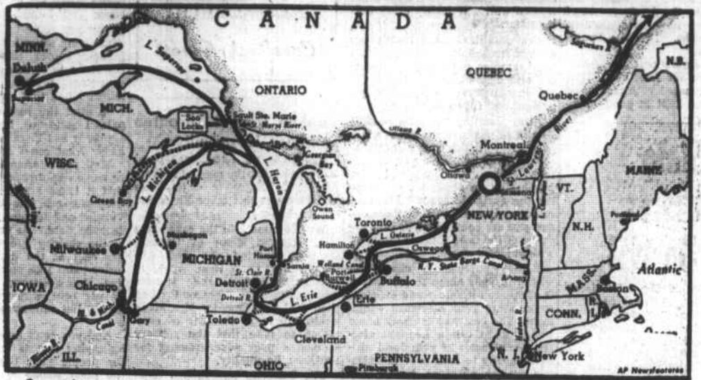
Ocean ships will sail far inland when St. Lawrence Seaway is completed. Project calls for building of 27-foot channel with canals and locks at International Rapids section of St. Lawrence River, shown in circle.
