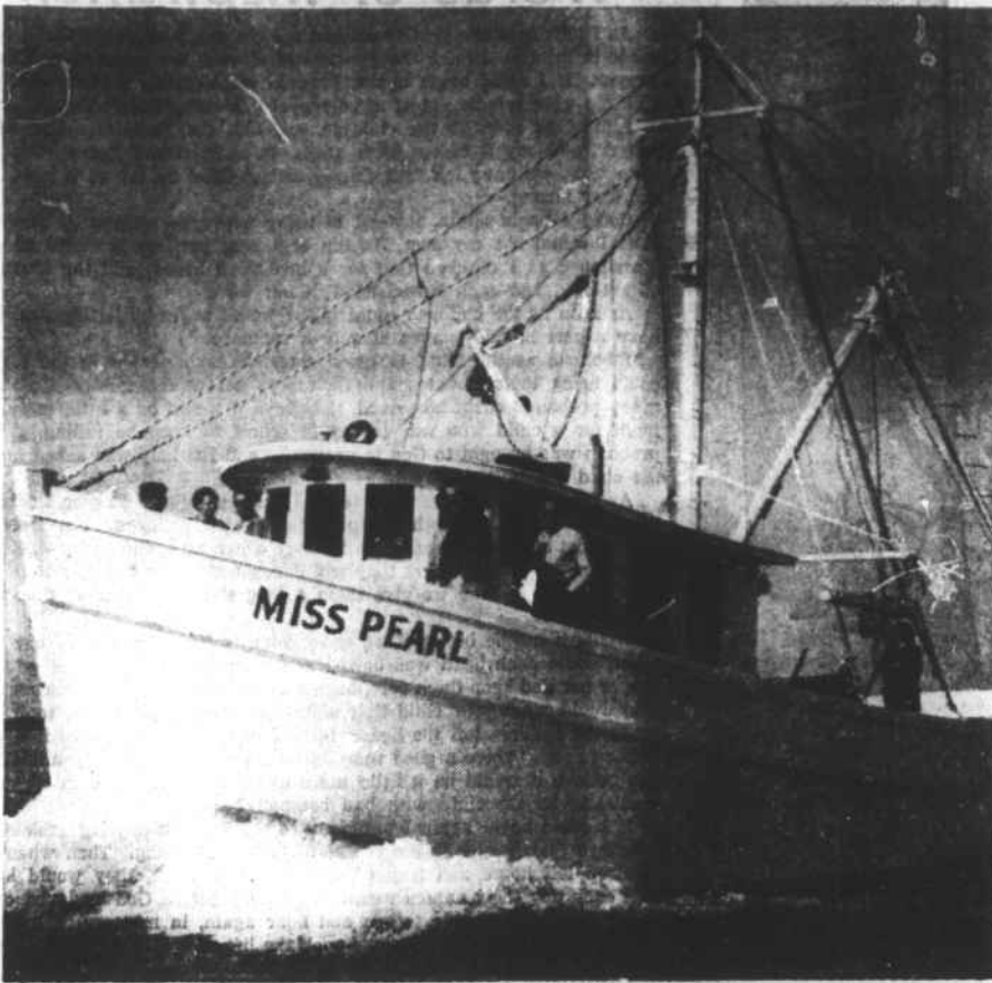
The Miss Pearl, 55-foot standard Hatteras trawler recently delivered to V. J. O'Neal of Morehead City, operator of one of Eastern North Carolina's better known fishing fleets. The boat was built by the Morehead City Shipbuilding Corp.
