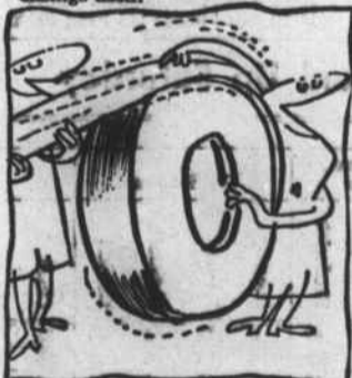
3. Thick band of new tire rubber banded to casing, sidewall to sidewall.
