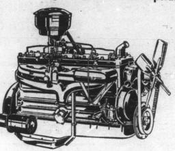
In Ford Series F-6—110 Horsepower, 212 lbs.-ft. Torque In Ford Series F-6 COE—106 Horsepower, 210 lbs.-ft. Torque
