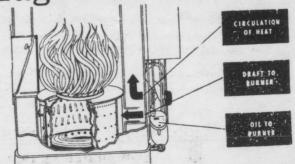
This simplified drawing shows how the Monogram burner works. As the oil flows to burner it turns into gas. Fan provides the draft and also circulates warm air to all corners of the home. No complicated gadgets or controls.
