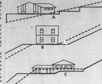
(A) A ranch-style house could not be constructed on the original grade indicated by the dotted line. Terracing the slope gives adequate space for
