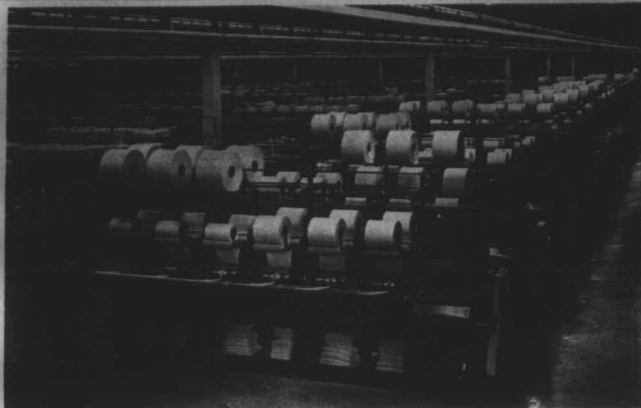
COMBING - Removes short fibers. Lays long fibers parallel
