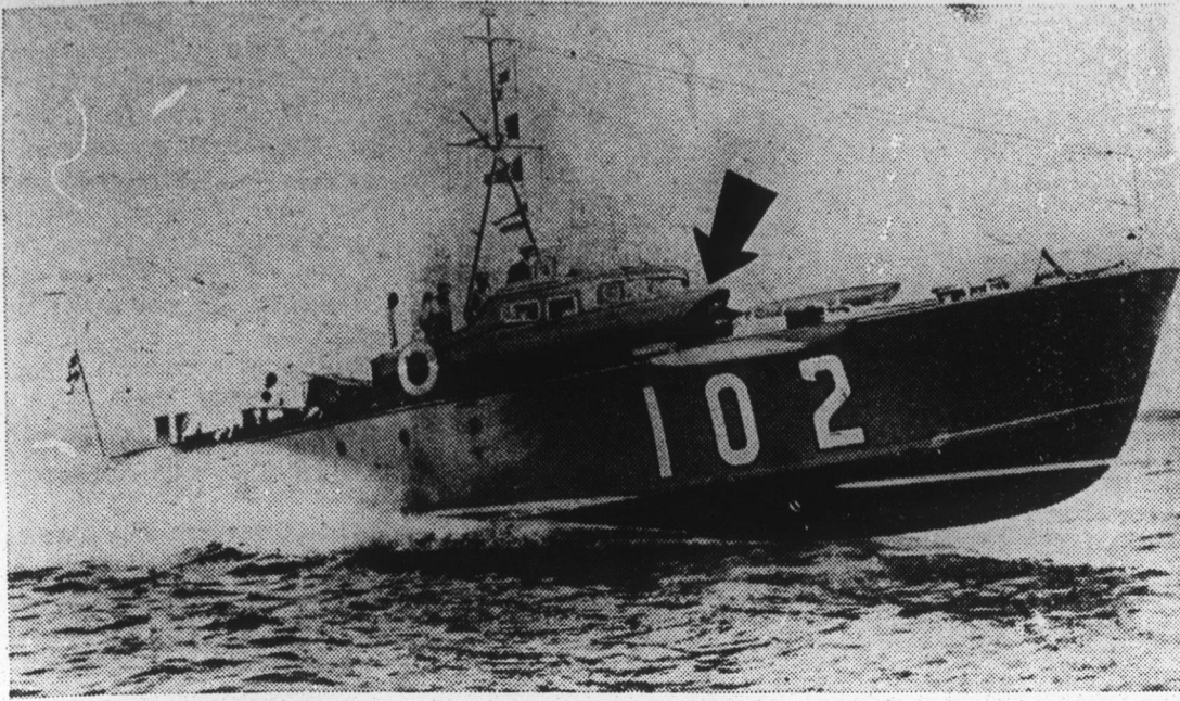
Here's one of Great Britain's powerful new torpedo boats which can launch a projectile straight ahead while traveling at top speed. Arrow points to one of the torpedo tubes mounted on deck. The British count on these boats to combat the German submarine. A large fleet of these boats has been placed in service in the North sea and they are usually attached to destroyer squadrons.
