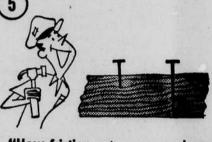
"How friction eats up power: longer nail is harder to remove, due to greater friction between wood and nail.
