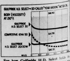
See how Gulfpride H.D. Select holds 13 "body" (viscosity). This new oil contains no artificial thickeners that break down under heat and pressure. But note how quickly a typical multi-viscosity 10W-30 oil starts to lose its body.
