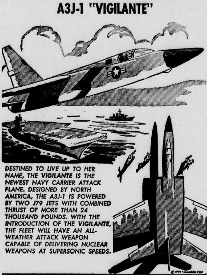
A3J-1 "VIGILANTE" DESTINED TO LIVE UP TO HER NAME, THE VIGILANTE IS THE NEWEST NAVY CARRIER ATTACK PLANE. DESIGNED BY NORTH AMERICA, THE A3J-1 IS POWERED BY TWO J79 JETS WITH COMBINED THRUST OF MORE THAN 24 THOUSAND POUNDS. WITH THE INTRODUCTION OF THE VIGILANTE, THE FLEET WILL HAVE AN ALL-WEATHER ATTACK WEAPON CAPABLE OF DELIVERING NUCLEAR WEAPONS AT SUPERSONIC SPEEDS.
