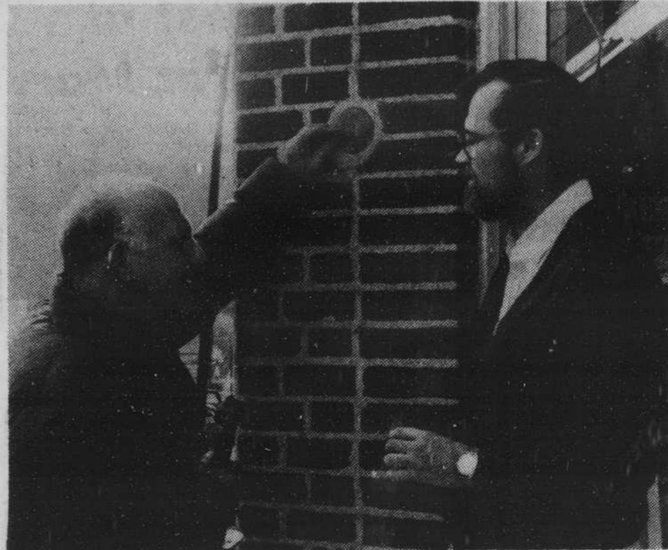
Steve Roberts, right, assists Bob McMeans in stamping the elevation on the bench mark on Black Mountain Drug Co.
