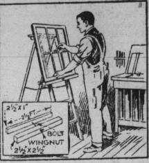
about 21/2 ft. long, with a bolt passing through the center of both as shown; a winguut is provided on the bolt. It is not necessary to remove the wingnut to attach the clamp. / Merely push the clamp over one leg of the stepladder from the inside, and then over the other leg, after which the wingnut is tightened. This tool can be used equally well on a common ladder.
