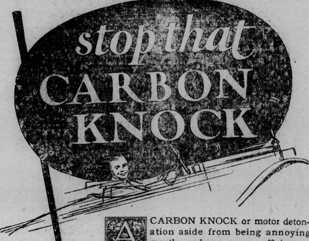
CARBON KNOCK or motor detonation aside from being annoying greatly reduces power efficiencycombustion taking place before the complete rise of the piston. The mechanical method of correcting such knocks is to retard
