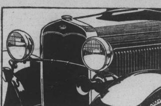
Bright, enduring RUSTLESS STEEL is used for many exposed bright metal parts of the Ford
