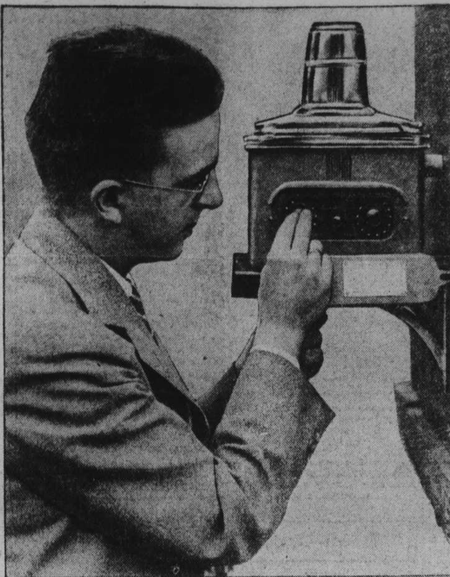
Left: The Electric Eye Which Controls the Light in a Trap for Exterminating by Electrocutation Moths and Destructive Bugs That Attack Crops. Above: Inspecting the Light Trap Which Electrocutates Moths and Other Insects. The Light Within Lures the Unsuspecting Bugs, Which Die Instantly on Coming in Contact With the High-Voltage Wires Around the Light. The Dead Insects Are Collected in the Pan.
