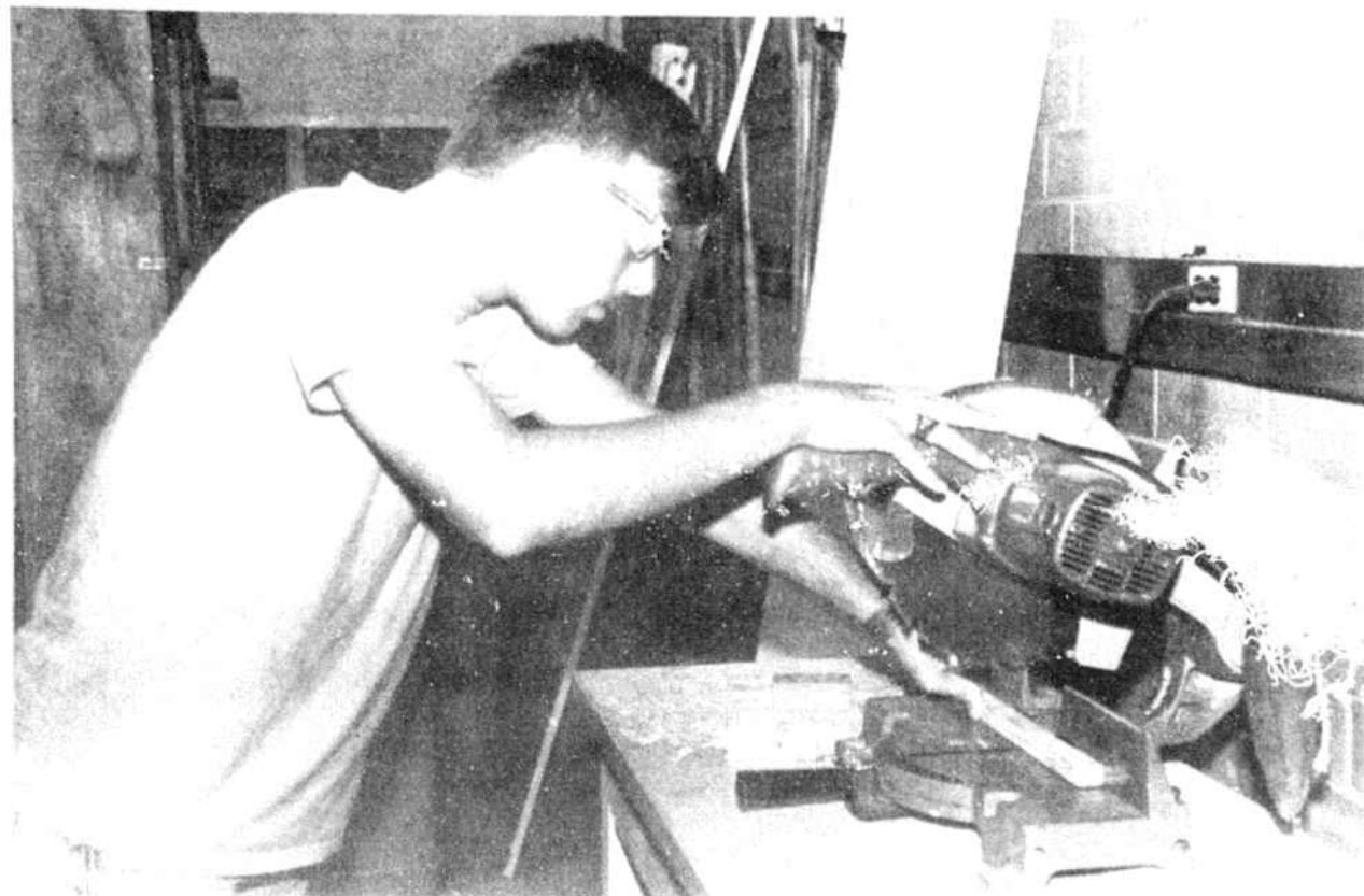
CHRIS THOMPSON, a Carpentry II student and Carpentry I shop assistant, cuts plywood for the sides of a truck's cargo area.
