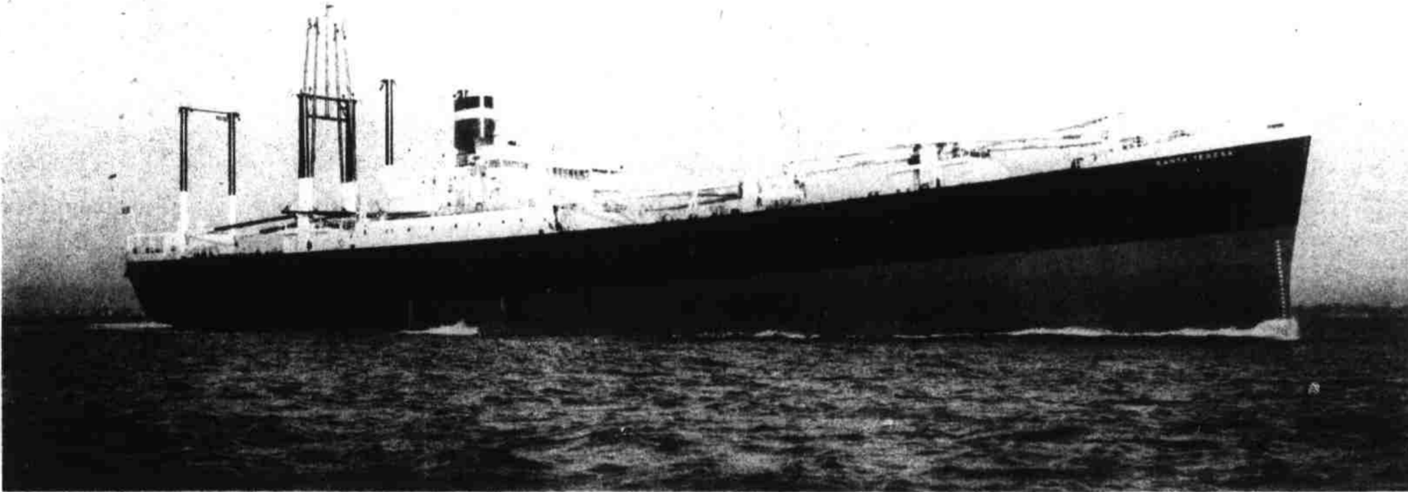
THE C-2—Nearing completion of its first three contracts for a total of 90 Liberty ships, the yard is now preparing to fulfill contract for 60 of the C-2 type vessels, similar to the one shown above. The ship, propelled by steam turbines, has a speed in excess of 14 knots and is somewhat larger than the Liberty freighter.
