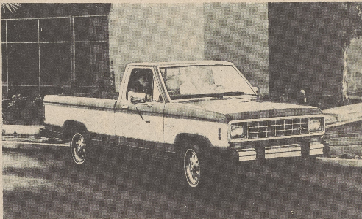
FOR WORK AND PLAY — The 1983 Ford Ranger brings to market the fuel economy you would expect from a compact truck, plus many of the attributes of the industry's most popular selling pickup — the full-size Ford F-Series. On the work side, Ranger offers big truck features such as Ford's Twin-I-Beam front suspension, half-ton-truck payload capacities, double-wall construction and body on ladder-frame construction. On the play side, Ranger can be fully equipped with appearance and power options and such comfort and convenience features as sporty bucket seats, plush carpeting, instrumentation, stereo radio choices and air conditioning. The Ranger is a featured attraction in Ford Division's exhibit at the 1982 World's Fair in Knoxville, Tenn., May 1 — Oct. 31.
