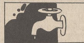
A faucet with its nozzle bent downward is called a bibcock.
