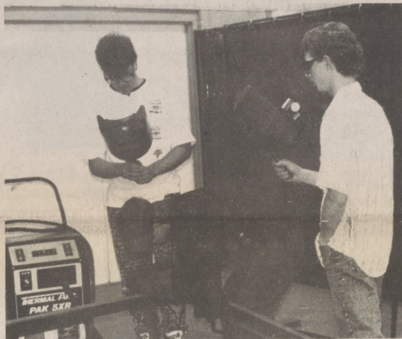
CLASSROOM OF THE FUTURE -Reese Cochran, left, Travis Withers and Mark Stacey demonstrate the new Plasma cutting system in Welding III at Kings Mountain High School. Welding instructor Tim Heavner, not pictured, says the new equipment cuts metal up to five inches thick and five times faster than oxyacetylene cutting and in the future will be used in transportation, nuclear power and chemical industries.
