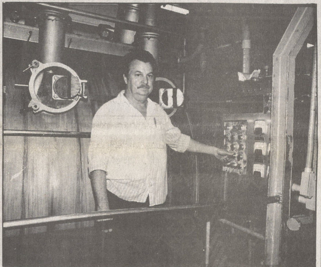
Jerry Williams operates the control panel on one of the Anvil Knitwear dyeing machines. Anvil is in the process of converting over to total automation. Their dyeing machines are computer-controlled, and are high-efficiency equipment. The coloring process is an integral part of Anvil's operation.
